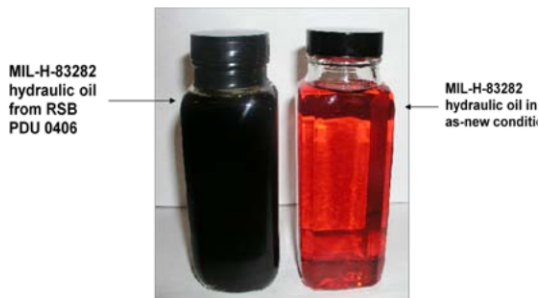
Figure 16: RSB gearbox oil comparison; new vs. old oil after 25 missions
