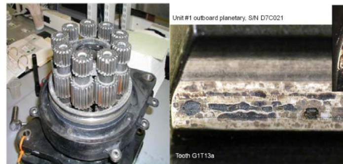
RSB actuator planetary gear corrosion damage
