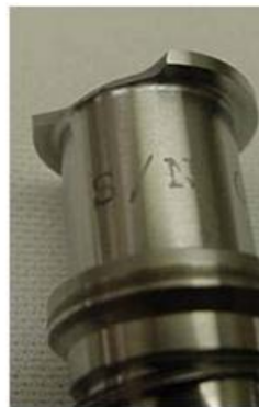
STS-126 broken FCV
