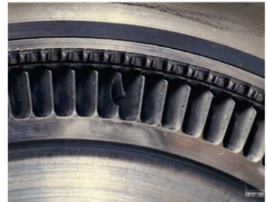
Figure 4: Close-up of fractured APU turbine blade
