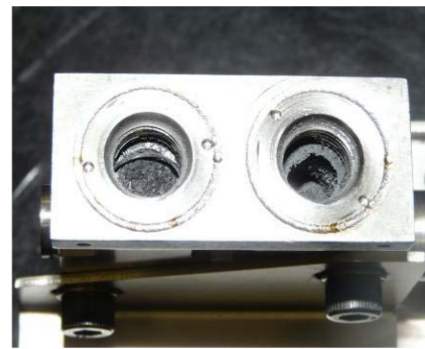
Figure 34: Pyrovalve (post-fire) showing result of failure.
