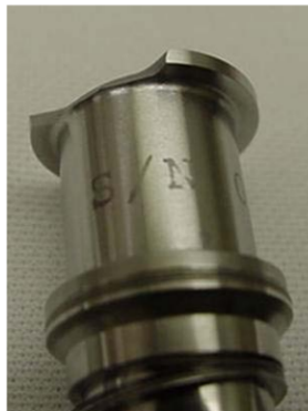
Figure 20: STS-126 broken FCV poppet
